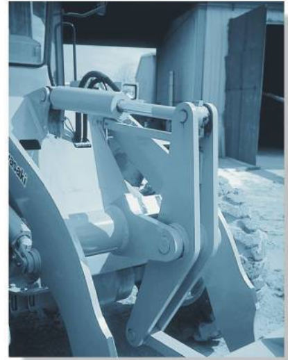
Many machine elements are pin connected in order to enable free rotation at their connections. These supports exert a force on a member, but no moment.
