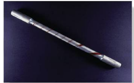
Severe twist of an aluminum specimen caused by the application of a plastic torque.
