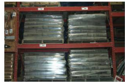
For safety, the beams supporting these bags of cement must be designed for strength and a restricted amount of deflection.
