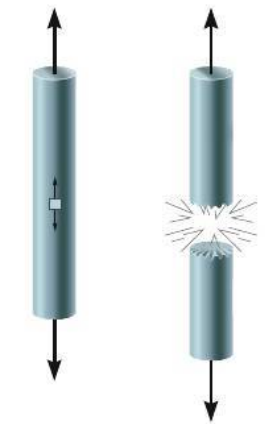
Failure of a brittle material in tension
