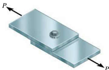
The area of the bolt for this lap joint is determined from the shear stress which is largest between the plates.
