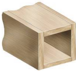
Wooden box beam
