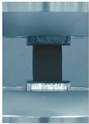
The rubber specimen is constrained between the two fixed supports, and so it will undergo plane strain when loads are applied to it in the horizontal plane.
