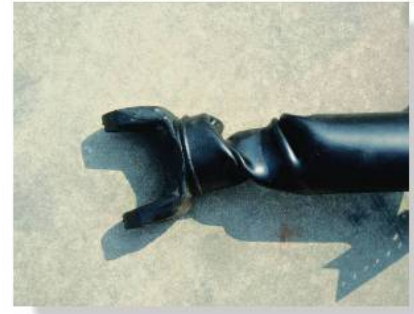
The tubular drive shaft for this truck was subjected to an excessive torque resulting in failure caused by yielding of the material. Engineers deliberately design drive shafts to fail before torsional damage can occur to parts of the engine or transmission.
