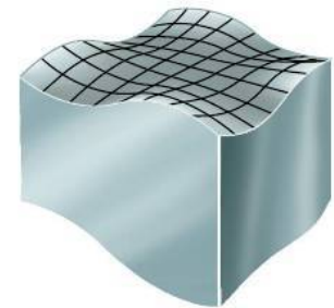
Warping of cross-sectional area
