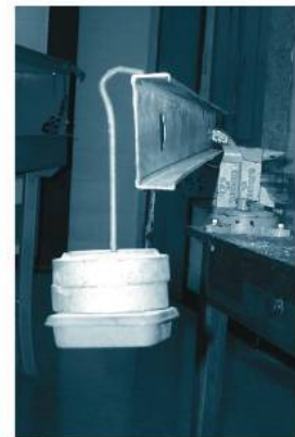
Notice how this cantilever beam deflects when loaded through the centroid (above) and through the shear center (below).
